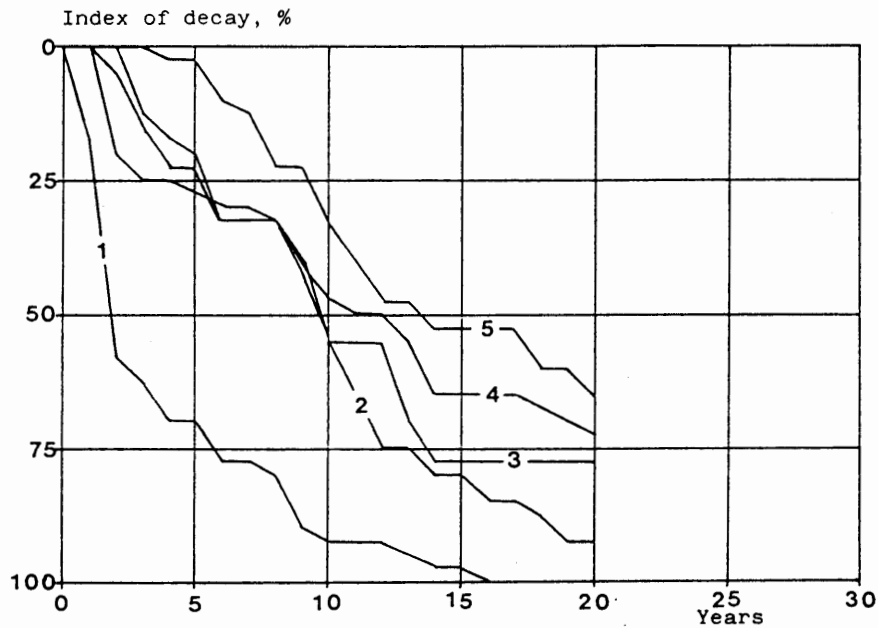
Figure 24. Rate of decay for stakes of European birch treated with Wolmanit CB at the following retentions (kg/m 3 ): 1, 8.8; 2, 13; 3, 18; 4, 27; 5, 36.
