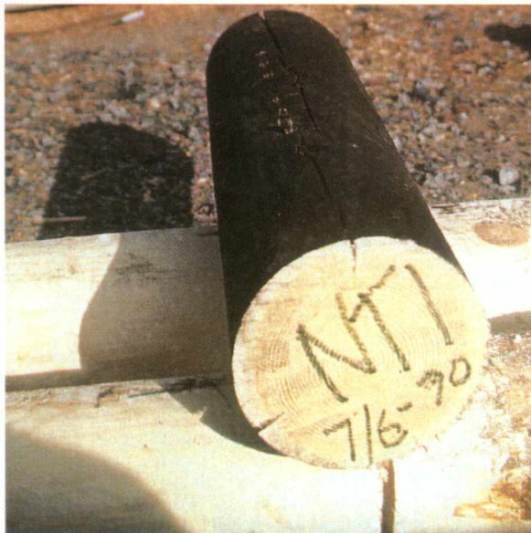
Figur 32. Stolpe utsatt for sooting ved røkgass-tørking i barkfyringsanlegg Figure 32. Poles dried in combustion gas. Sooting caused by insufficient combustion
