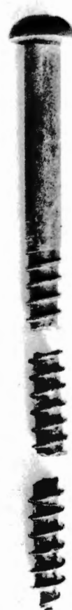
Bild 4. Mässingsskruv med 2 brott pga spänningskorrosionsprickning. Stress corrosion cracking has caused the breakage of this brass screw.
