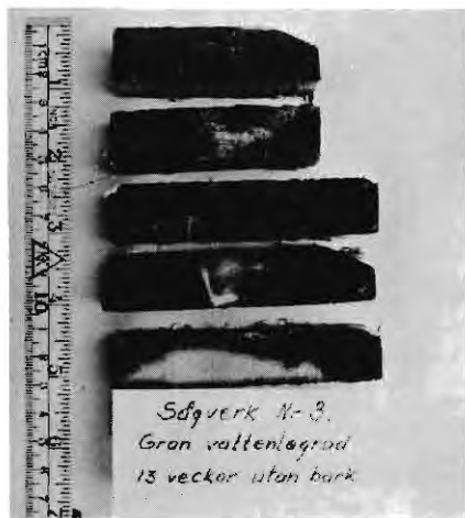
Fig. 9. Water-storage for 13 weeks, sawmill no 3. Nearly complete penetration.
