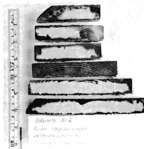
Fig. 8. Water-sprinkling of barked logs on land for 20 weeks, sawmill no 6. Incomplete penetration.
