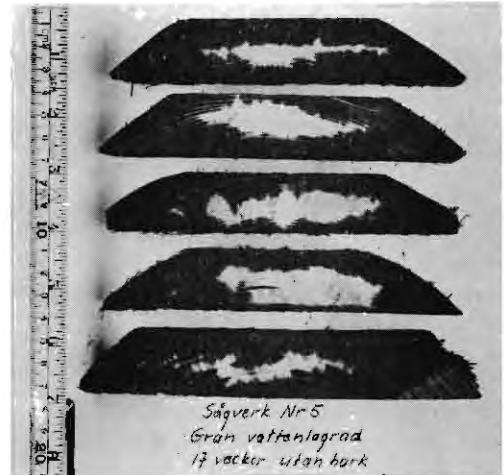
Fig. 2. Water-storage of barked logs for 17 weeks, sawmill no 5. Incomplete penetration but better than for controls (see fig. 1)
