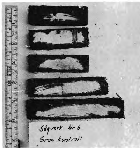
Fig. 3. Controls from sawmill no 6. Incomplete penetration.
