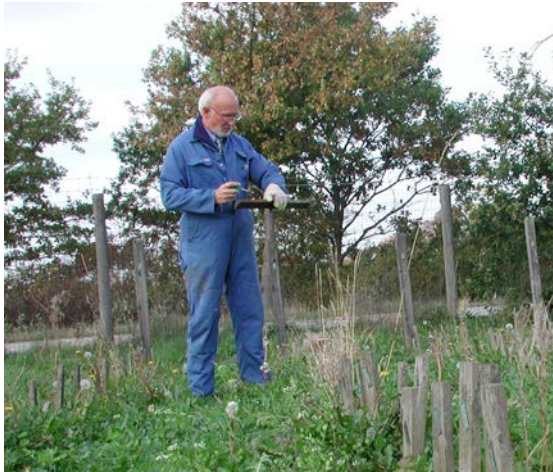
Figure 3. Inspection of EN 252 stakes by Mr Keld H Henriksen at Tåstrup (left) and Mr Fred G Evans at Sørkedalen (right).
