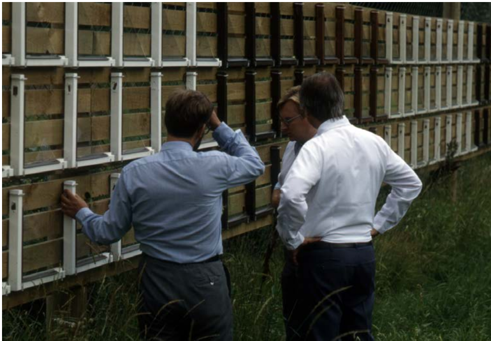
Figure 6. Mr Eero Kangas (middle), former Director of the Finnish Wood Preserving Association, demonstrates L-joint testing at the Viikki test site.
