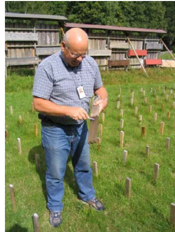
Figure 3. Inspection of EN 252 stakes by Mr Keld H Henriksen at Tåstrup (left) and Mr Fred G Evans at Sørkedalen (right).
